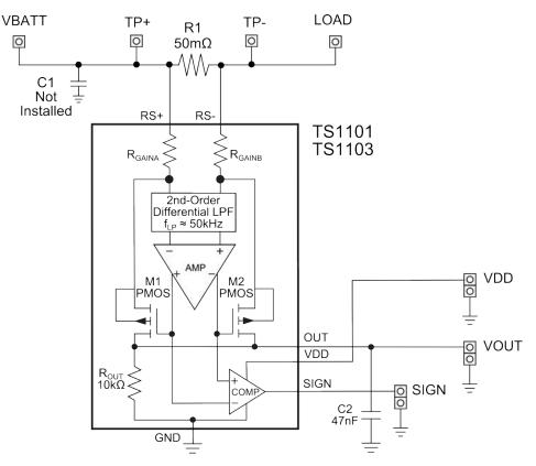
Figure 4.1. TS1101/03DB Demo Board Circuit Schematic
