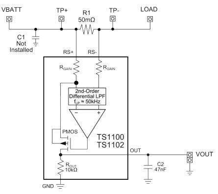
Figure 2.1. TS1100/02 Demo Board Circuit Schematic
